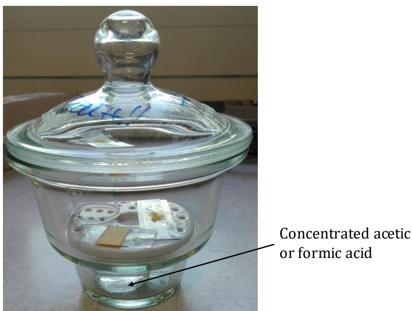
Fig.9 – Experimental set-up for the exposure of the pigments to acetic and formic acid
