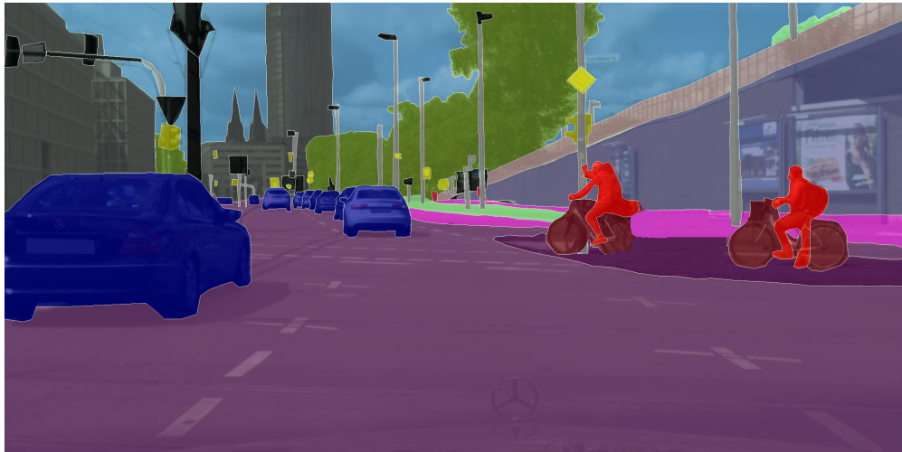
Figure 3.6: Segmentation obtained by injecting adversarial noise.
