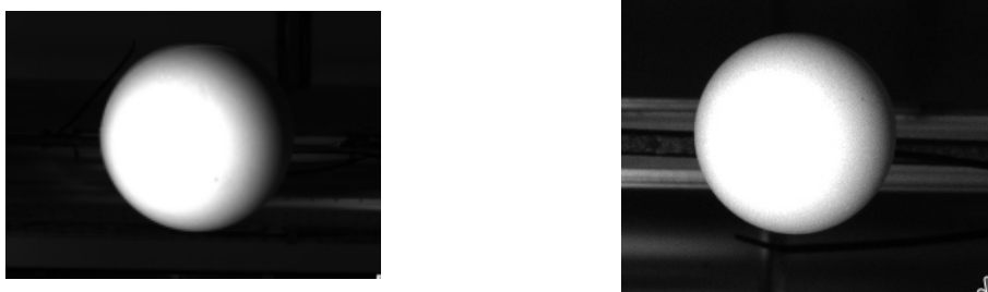
Figure 6.7: An example of why the big ball fitting is slightly more imprecise with respect to the small case. On both image, the ball is placed in its position farthest away from camera. While in the small ball the contour is clearly visible, in the big one it is obscured and might be estimated poorly
