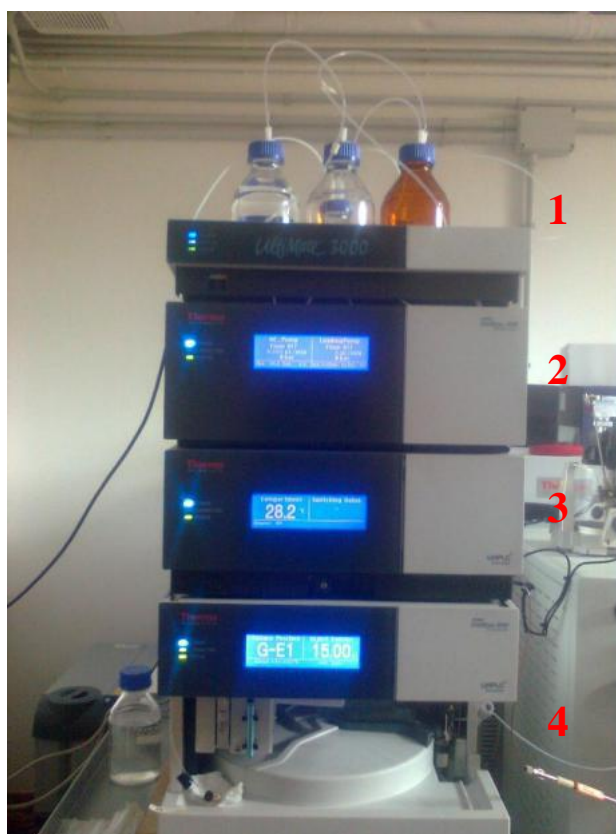
Figura 15: l'UHPLC™ (Ultra High Performance Liquid Chromatography) UltiMate 3000 (Thermo Fisher Scientific™).
