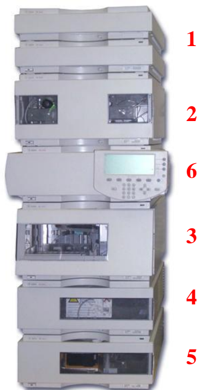
Figura 16: HPLC™ (High Performance Liquid Chromatography) Agilent 1100 (Agilent, Waldbronn, Germania) [Agilent Technologies, 1999]
