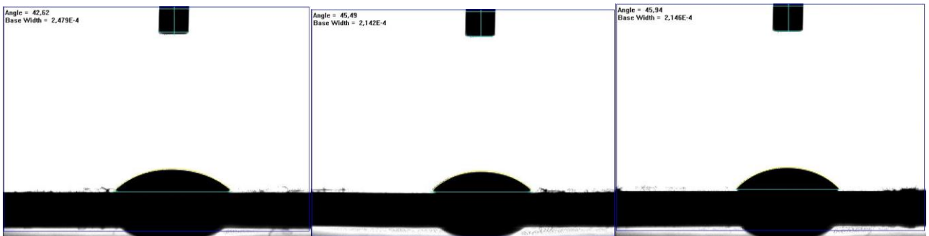
Diiodomethane contact angle diagrams of Sample 3 (first category of samples)
