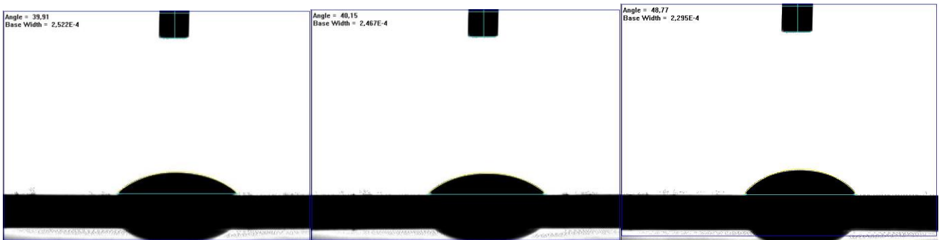
Diiodomethane contact angle diagrams of Sample 2 (first category of samples)
