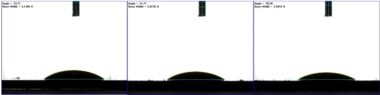
Diiodomethane contact angle diagrams on sample 1 (first category of samples)
