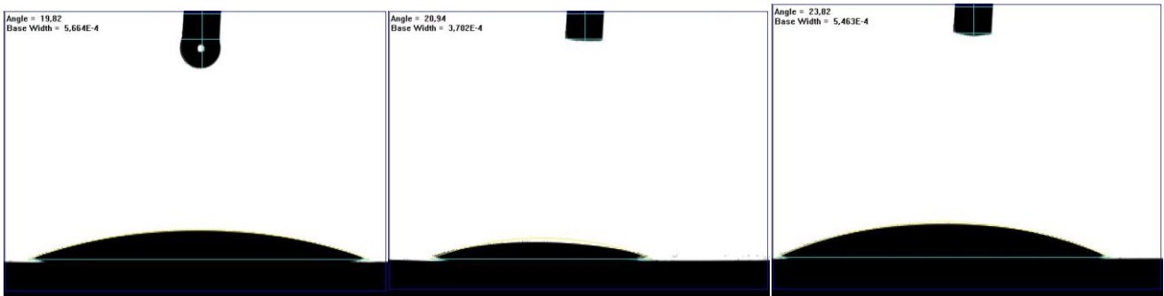
Water contact angle diagrams of Sample 4 (first category of samples)
