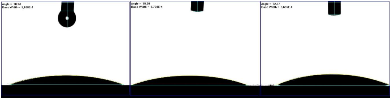
Water contact angle diagrams of Sample 6 (first category of samples)
