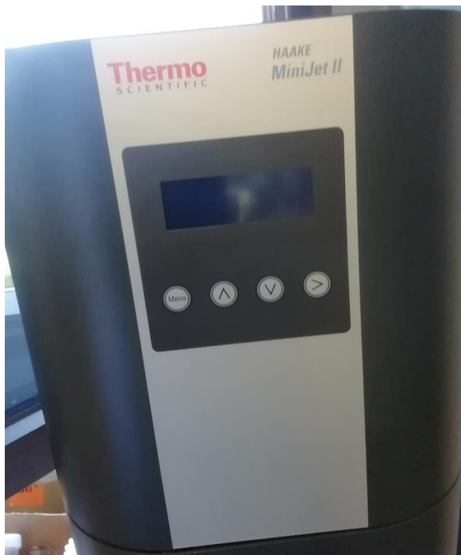
Figure 20/ Haake MiniJet II used to prepare the polymer substrates
