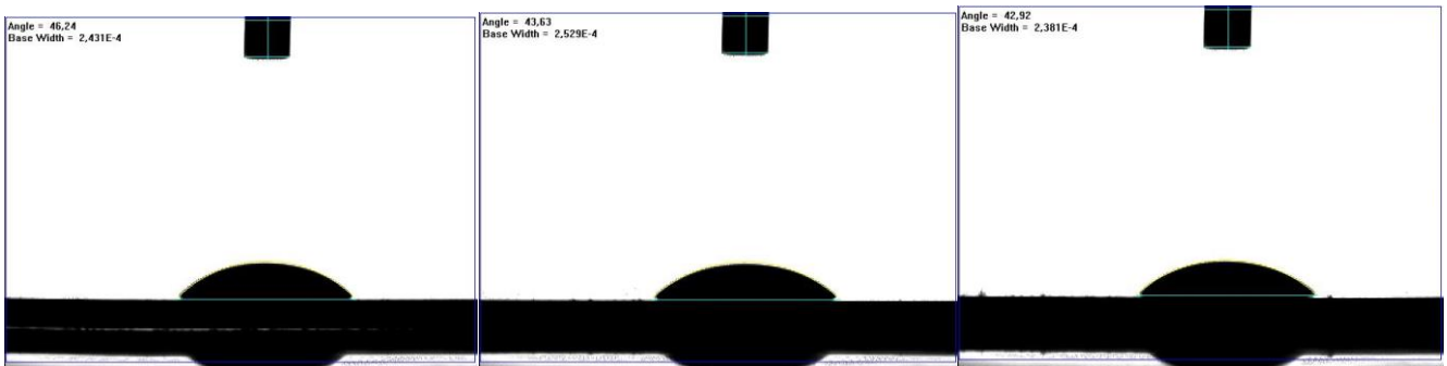
Diiodomethane contact angle diagrams of Silicon wafer as the reference
