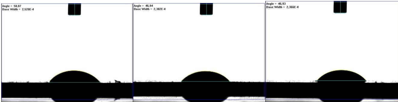
Diiodomethane contact angle diagrams of Sample 9 (first category of samples)
