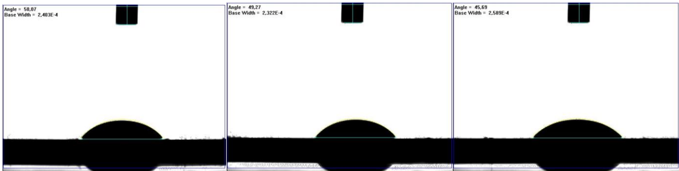
Diiodomethane contact angle diagrams of Sample 6 (first category of samples)
