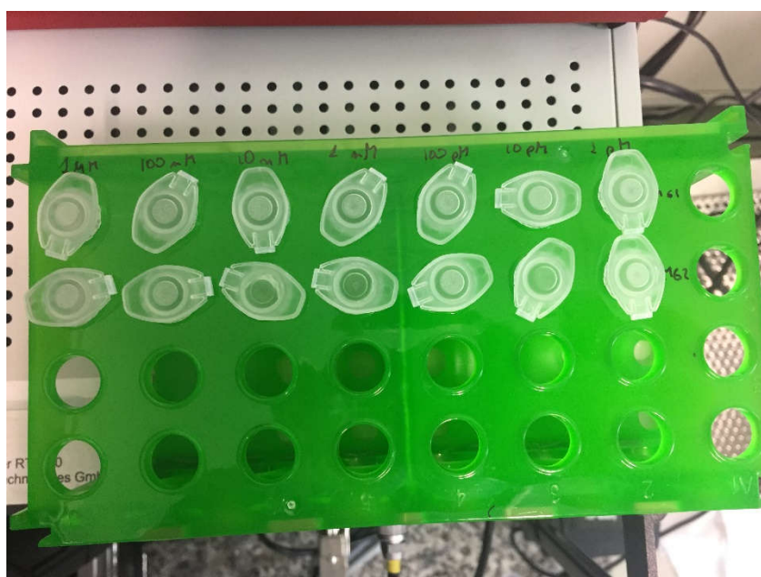
Figure 48. Tube rack holding the tubes organized with descending concentration from 1\ \mu\text{M} to 1\ \text{pM}
