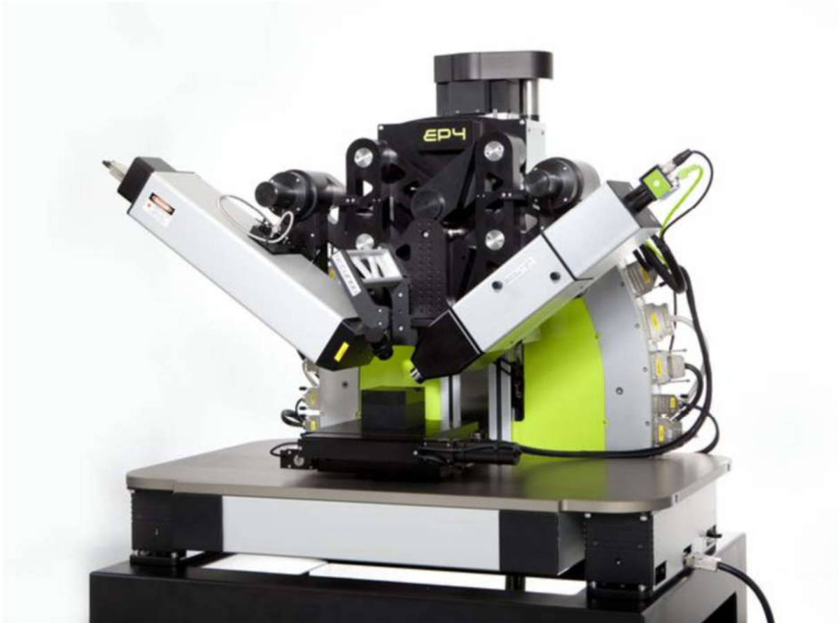
Figure 17. Nulling ellipsometer Nanofilm-EP4 employed in the present thesis work.
