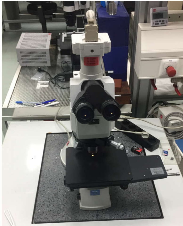
Figure 19. Nikon Eclipse L150 optical microscope used to acquire all the optical microscopy images.
