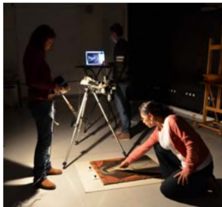
Figure 2.4: Conservators during data capture using the RTI Highlight method, where a light source is moved around the object and a new image is taken for each light angle [51]
