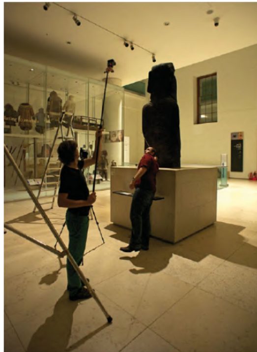
Figure 1.5: RTI capture, with the camera fixed on scaffolding just out of shot to left; light is delivered by moveable remote flash, set at a constant distance from the statue determined by a length of string. [8]
