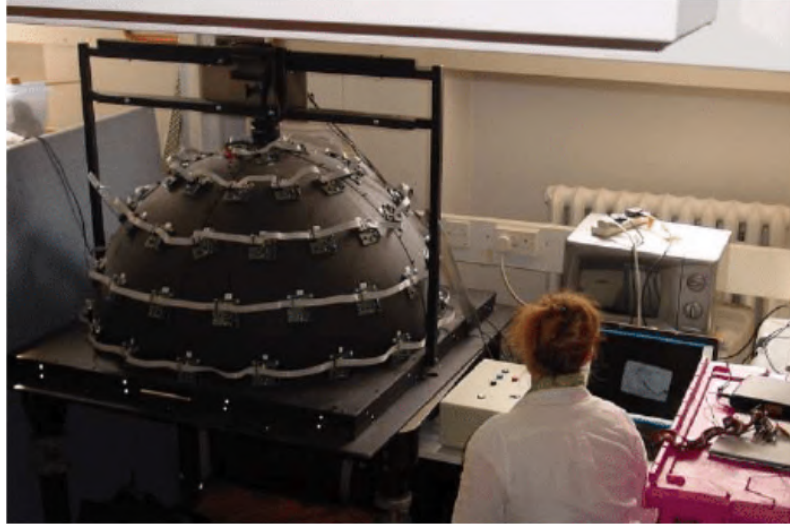
Figure 2.4: Conservators during data capture using the RTI Highlight method, where a light source is moved around the object and a new image is taken for each light angle [51]
