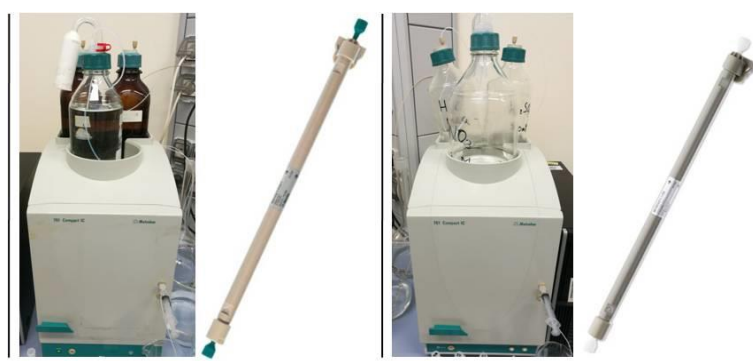
Figure 22 Chromatographs and column used for the anions (left) and cations (right) detection [82].
