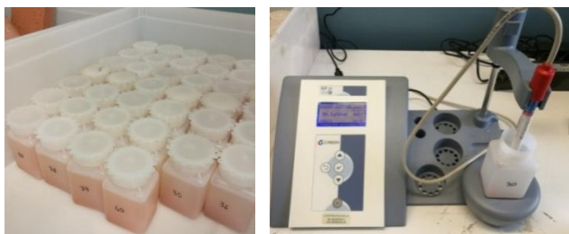
Figure 20 Sample solutions (left) and their conductivity measurements (right): conductometer and conductivity cell used.
