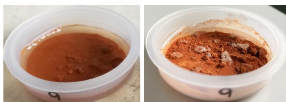
Figure 34 The formation of the water layer and subsequently of the salt crystals for the sample at 140 cm height and 0-
