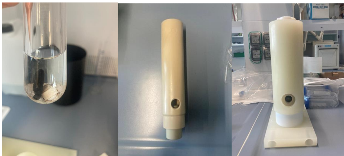
Figure 3.8: (Left) glassware in quartz filled with reagents and equipped with magnetic stirrer and black disk; (Centre) tube in PEEK; (Right) Teflon insert charged with tube PEEK and glassware closed with the appropriate cap.
