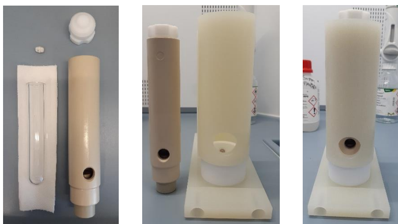
Figure 3.2. Microwave equipment. From left to right: quartz vessel with magnetic stirrer, PEEK cylinder with screw cap, Teflon support.
